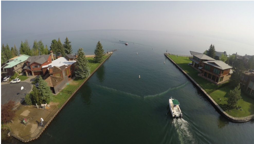
A bubble curtain as seen from a drone/League to Save Lake Tahoe
