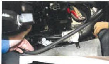
Ballast system water pump, water lines, and caps should all be flushed and cleaned.
