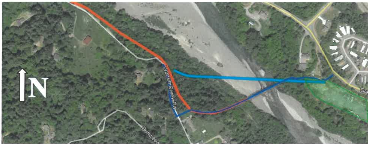
Figure 5 – Site map showing location of original water line and approximate trenchless alignment
