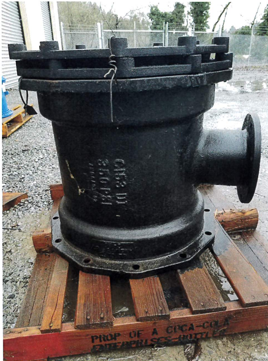
Sigma DG18, 350 psi class 18" Ductile Iron Tee, MJ x MJ x 6" flange Overall length 24" Estimated value new: $1,500.00
