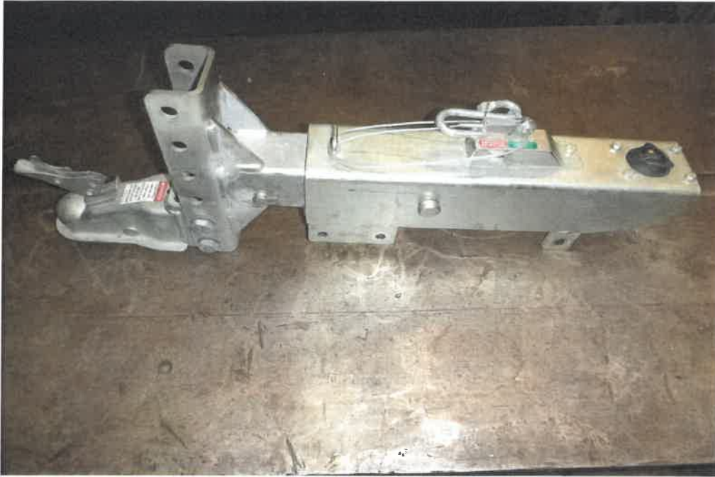
2" Demco Hydraulic brake actuator assembly #DA91; (2) 12" x 2" Hyd brake backing plate assemblies 5 bolt.
