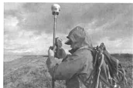
John Herrera uses a Trimble R10 Real Time Kinematic GPS units at Lanphere.
